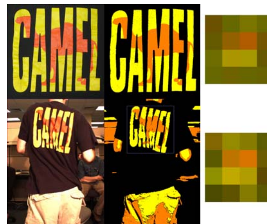
Fig. 7. Our method requires a frontal view of the texture ( top row ) and a target image ( bottom row ). We quantize the colors using a color classifier, then compute a 4 \times 4 color histogram, with separate bins for each color channel. In this case, with three colors (black, orange and yellow), our descriptor is 4 \times 4 \times 3 . We visualize this descriptor by reconstructing the colors and normalizing appropriately ( right ). A search for the descriptor in a subsampled version of the target image reveals the closest match ( bottom right ).
