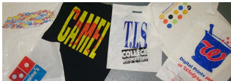
Fig. 1. Many common textured articles are made using screen printing — where each color is printed in a separate pass. Often, this method is cheaper than using a full color gamut. Screen printing is widespread: many T-shirts, advertisements, and corporate logos are composed of a small number of solid colors. Recovering irradiance is easier in this setting: correspondence to a frontal view of the pattern is not required. Instead, each color can be detected independently in order to recover irradiance. Because screen print items are composed of large regions of uniform color, they are robust to motion blur.
